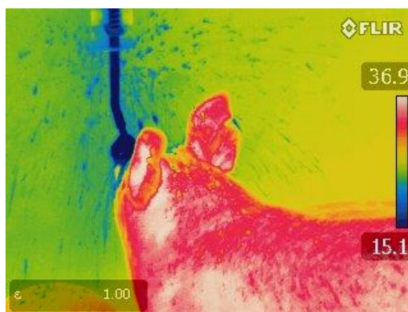
Figure 1.1. The infrared thermal image shows a heat stressed grow-finish pig drinking cool water from a nipple water drinker line affixed to the pen wall. The water droplets spraying from the waterer are lower in temperature than the surrounding walls and animal.
