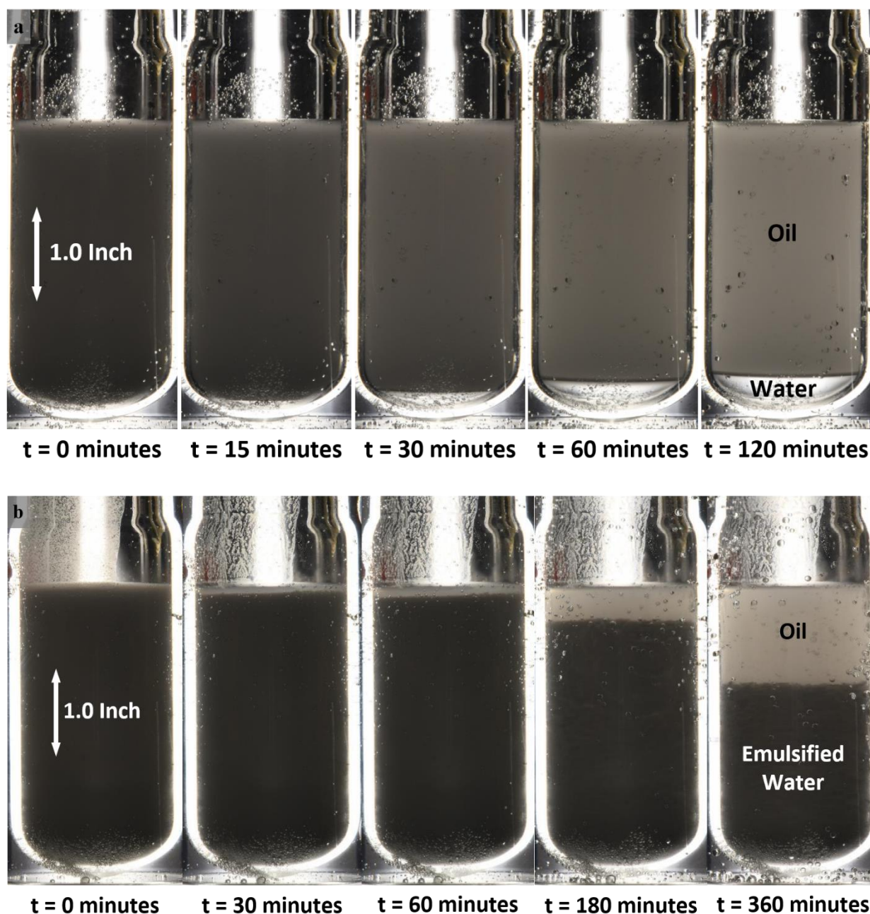
Fig. 3.3 Sample emulsions formed between water and squalane oil using different surfactants. a) Polyethylene glycol oleyl ether used as a surfactant. b) Sorbitan monooleate used as a surfactant.
