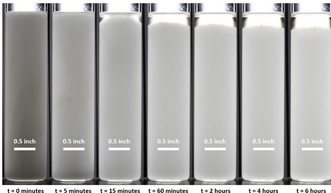
Fig. 4.34 Ethanol-in-paraffin oil emulsion formed with Span® 80 as surfactants. Composition is 85 wt.% oil, 10 wt.% aqueous ethanol solution, and 5 wt.% surfactant.
