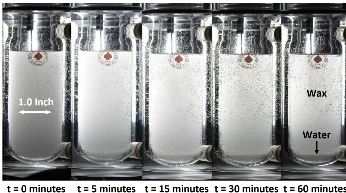
Fig. 4.13 Water-in-wax emulsion control group, formed without a surfactant. Composition is 90 wt.% wax and 10 wt.% DI water.
