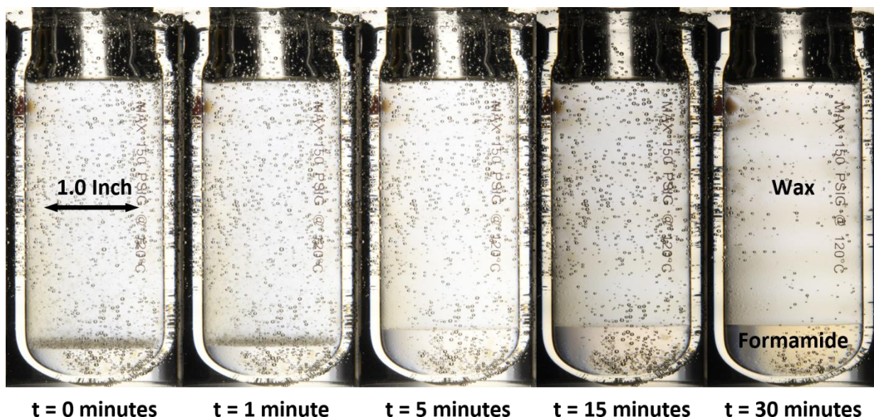
Fig. 4.20 Formamide-in-wax emulsion, formed with Span® 80 as a surfactant. Composition is 79.5 wt.% wax, 20 wt.% formamide, and 0.5 wt.% surfactant.
