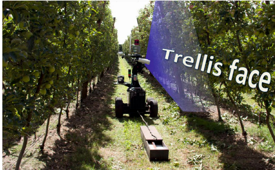
Figure 2.5. Research ground vehicle traversing between two trellis rows and scanning with LiDAR (Bargoti et al., 2015)
