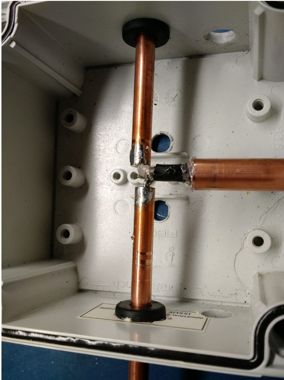
Fig. A.5.: Coax to Antenna Elements Soldering
