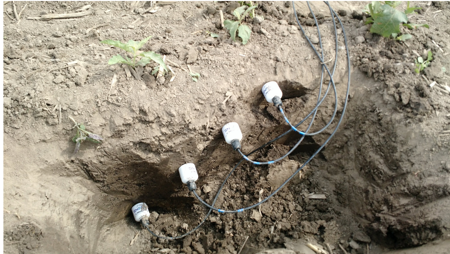
Fig. 4.14.: HydraProbe Installation - 2018 Field Experiment
