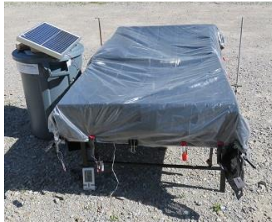
Figure 7.4 Drying test with the folding bed dryer
