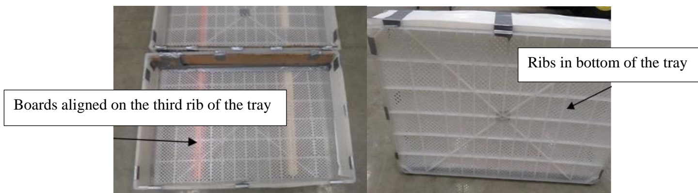
Figure 4.16 Boards aligned to support trays (left); bottom of Tray showing “ribs” that add strength to the trays (right)
