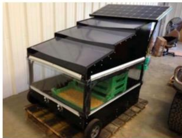
Figure 2.7 The forced convection solar dryer [34]
