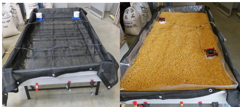
Figure 7.3 The folding bed dryer (left) prepared to receive the maize and (right) filled with maize
