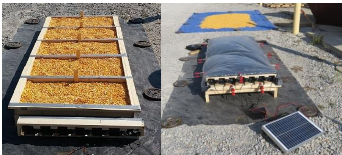
Figure 4.8 The 123 kg of maize in 5 wooden trays (left); maize drying in POD (foreground) and on a tarp (right background)
