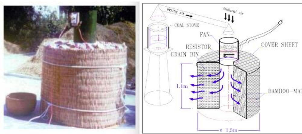
Figure 2.4 The SRR dryer developed by Nong Lam University in Vietnam [27]
