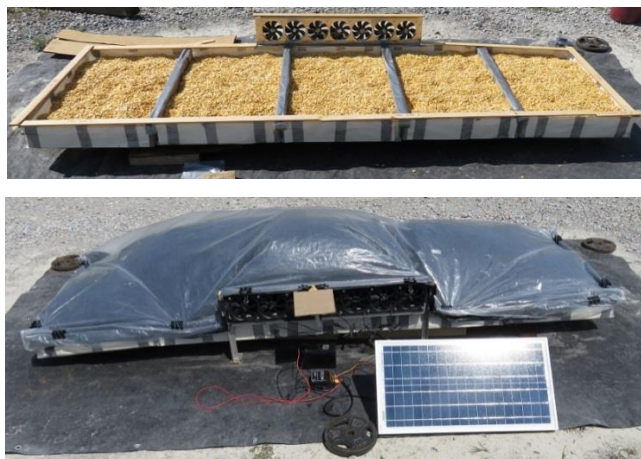
Figure 4.22 Modified POD that uses an aluminum fan frame
