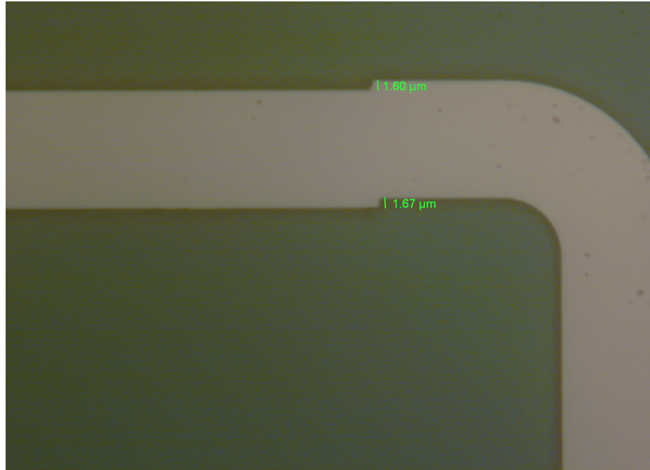
Figure 4.13. Stitch error in mask write during E beam lithography leading to poor mask definition.
