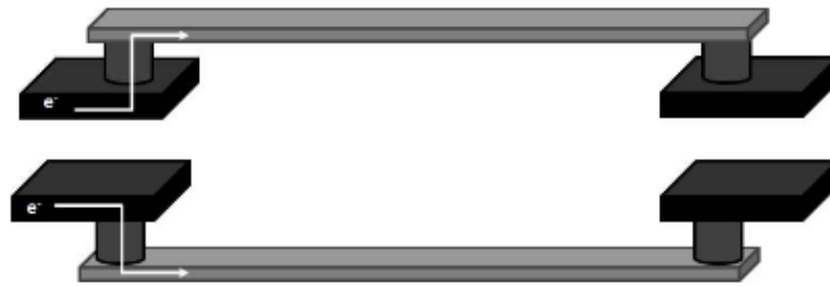
Figure 3.2. A line-via-line schematic for a test structure with two layers of metallization.
