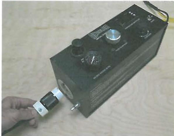
11. Connect compressed air to the base/power unit. Note: Compressed air supply must not exceed 150 psig (1,034 KPa).
