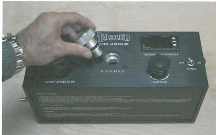
7. Using the supplied funnel, fill the fluid reservoir with an approved fluid. The fluid can be filled up to the bottom of the filler plug threads.
