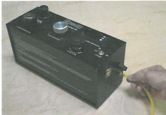
3. Connect the wand power cord to the base/power unit.
