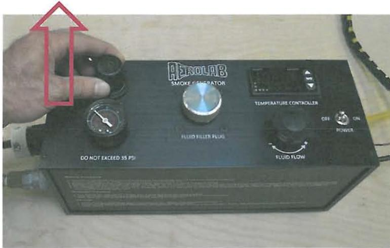
13. While watching the air pressure gauge, turn the **PRESSURE REGULATOR** knob clockwise or anticlockwise to adjust the reservoir pressure to 20 psig.
