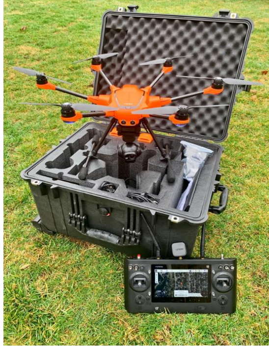
Figure 2: Yuneec H520 UAV, CGOET camera, and ST16S ground control station.
