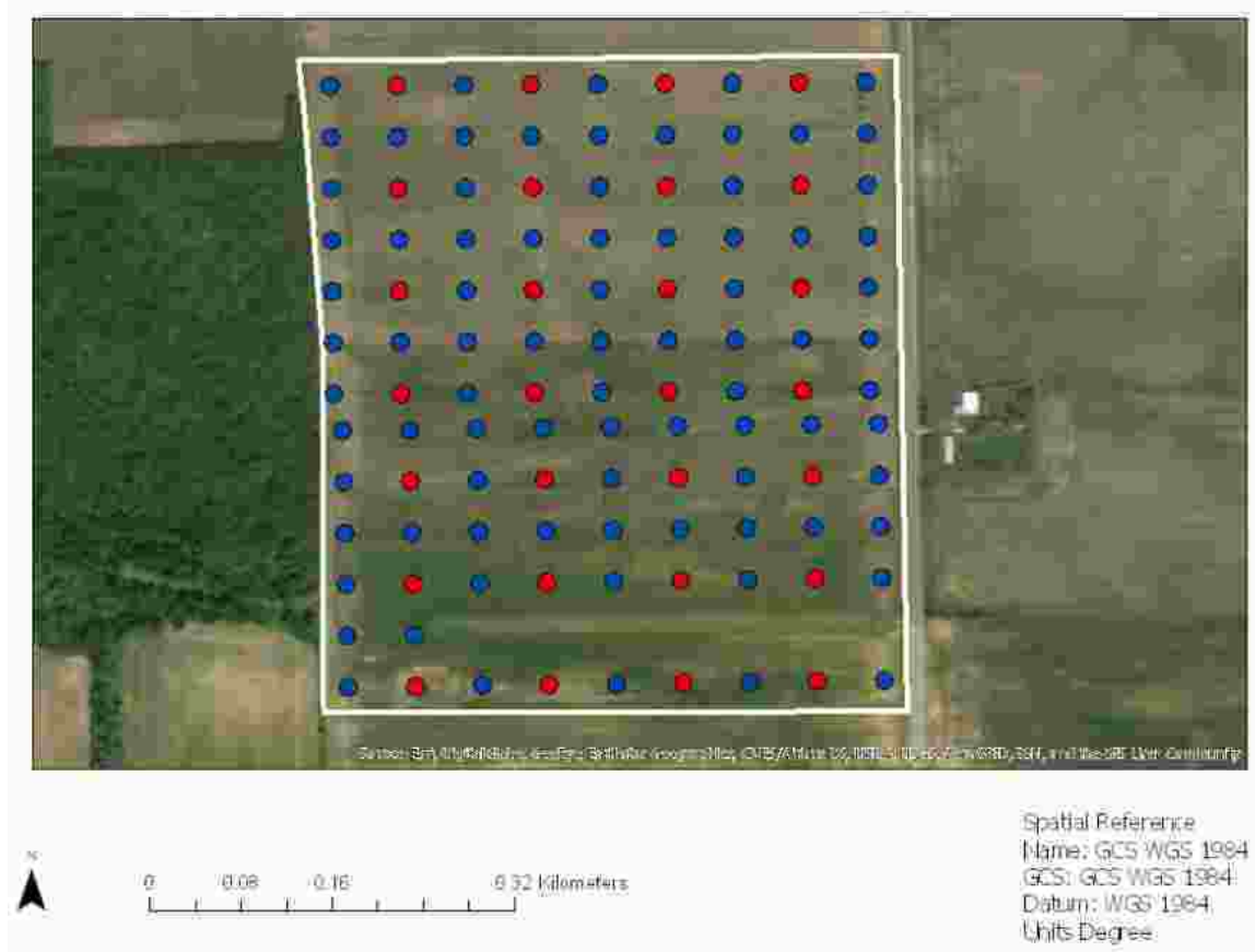
Figure 3.3.: Points Selected For Training, Validation Points, and Site Boundary. Points Selected For Interpolation are Displayed in Red, While Points Kept For Validation are Displayed in Blue.
