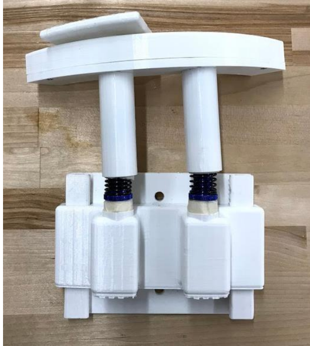
Figure 2.9. First Sliding Track Prototype. (Corens, Jakub, Pessler, & Wigren, 2018)
