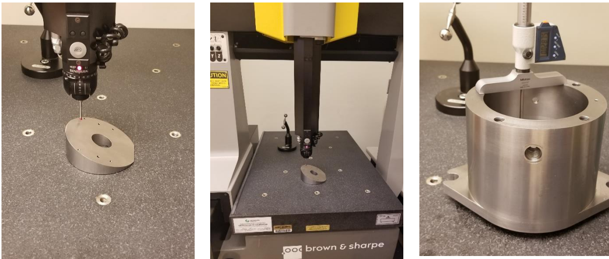
Figure 8.2. CMM inspection of components.
