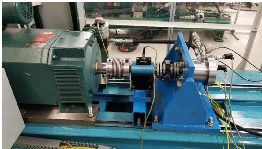
Figure 8.12. Steady state test rig with 24 cc prototype mounted.
