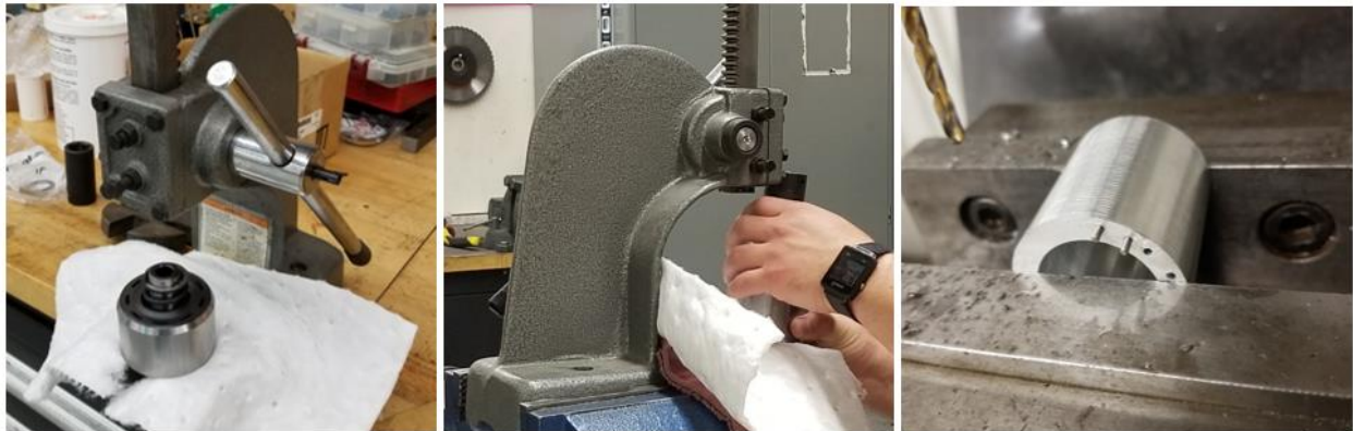
Figure 8.11. Fixture to install cylinder block spring and snap ring.
