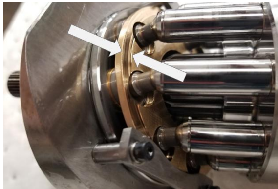
Figure 9.13. Worn slipper retainer plate after measurements.
