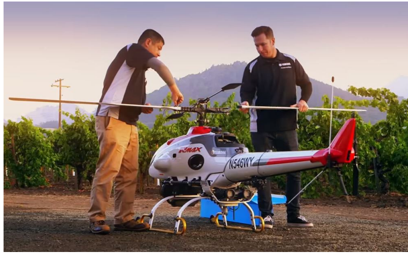
Figure 2.13. Setting up Yamaha R-MAX for Custom Herbicide Application in Vinyard, Sonoma Valley, CA ( Yamaha Motors USA, 2016 ).
