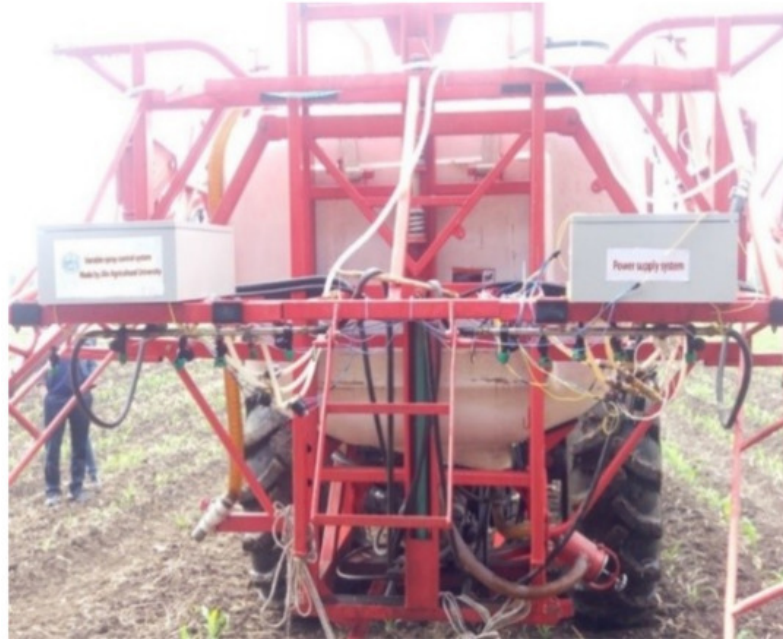
Figure 2.9. Xu et al. (2018)’s Smart Sprayer System Configuration.
