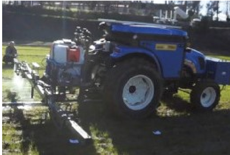
Figure 2.12. Gonzalez-de-Soto et al. (2016) 's Unmanned, Herbicide-applicator Robot, Based off of New-Holland Tractor.
