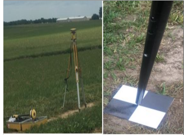
Figure 3.7. TopCon HiPer V™ RTK Base Station and Receiver and GCP Measurement.
