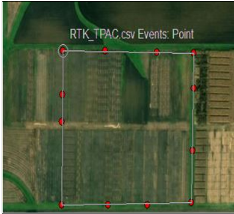
Figure 3.6. Ground Control Point Boundary Map Created from RTK Point Collection.
