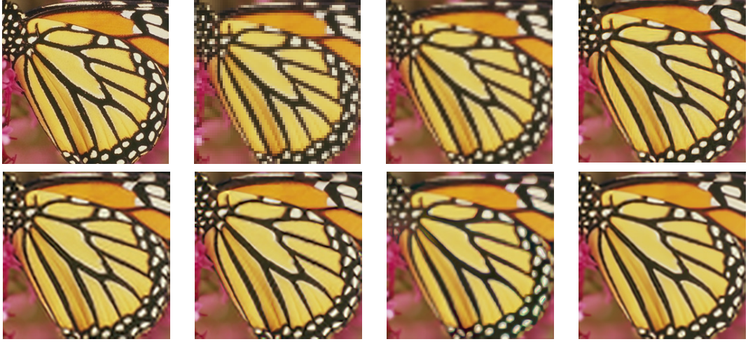
Fig. 3.8.: Image Super Resolution Results. [Top](from left to right). Ground truth; The low resolution input; Bicubic interpolation; DCNN [49] (24.19dB). [Bottom](from left to right). SPSR [50] (22.44dB); TSE [86] (22.80dB); GPR [51] (20.81dB); Ours-M (23.49dB).
