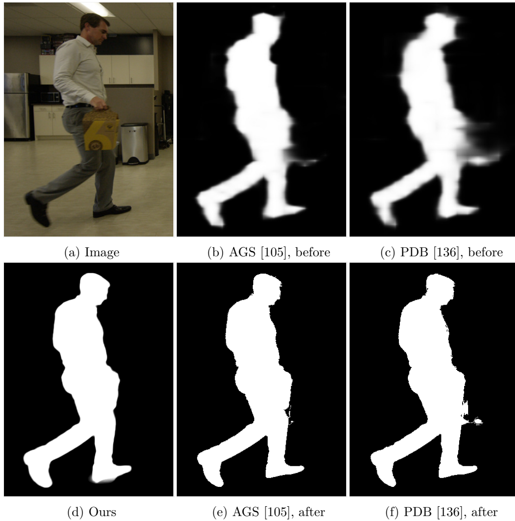
Fig. 5.11.: Dependency of conditional random field. (a) Input. (b) Raw output of the neural network part of AGS [105]. (c) Raw output of neural network part of PDB [136]. (d) Our result without post-processing. (e) Post-processing of AGS using conditional random field. (f) Post-processing of PDB using conditional random field. Notice the rough raw output of the deep neural network parts.
