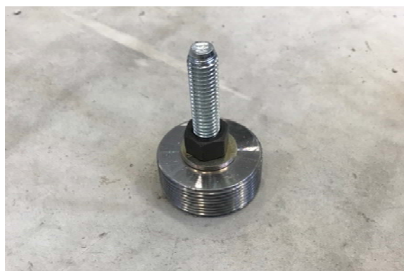
Figure 3.5: Torque-controlled anchor expansion after being installed in concrete specimen
