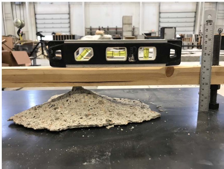
(a) Upside-down concrete breakout cone
