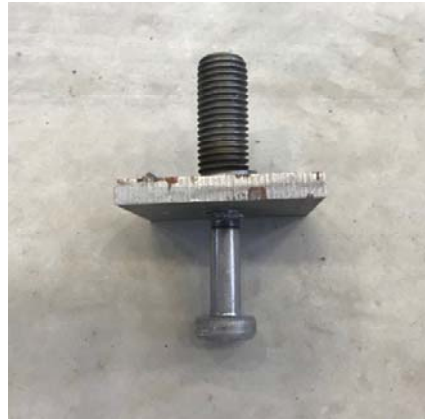
Figure 3.8: Cast-in anchor after tension test
