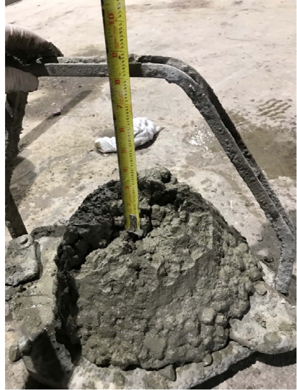
(b) Slump test
