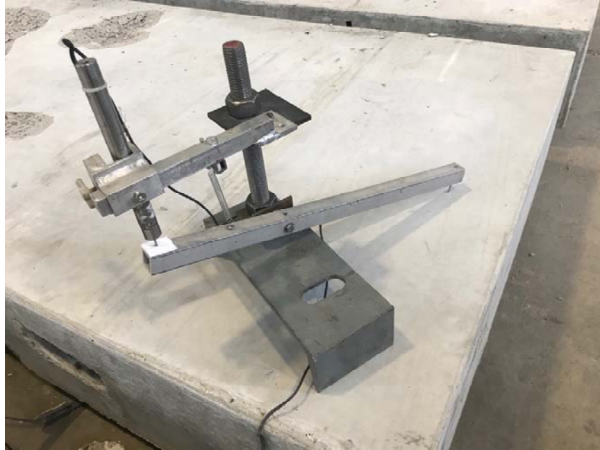
Figure 3.13: Displacement measuring device
