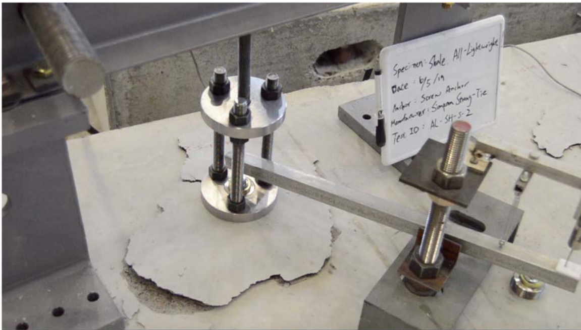
Figure 3.14: Displacement measuring device after failure of an anchor
