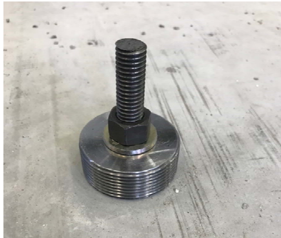
Figure 3.6: Displacement-controlled expansion anchor after being installed in concrete specimen
