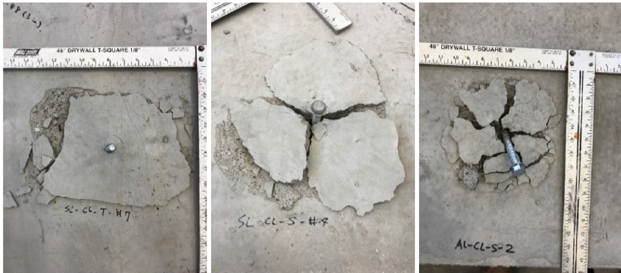
(a) Typical concrete breakout
