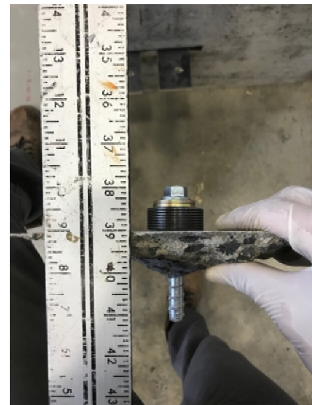
(b) Concrete breakout cone of screw anchor
