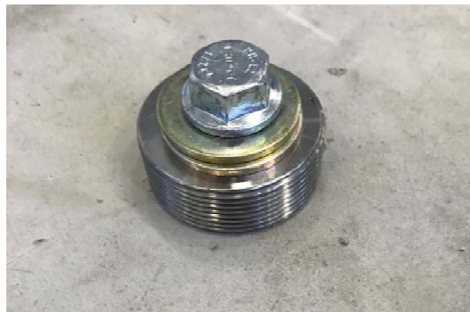
Figure 3.7: Screw anchor after being installed in concrete specimen
