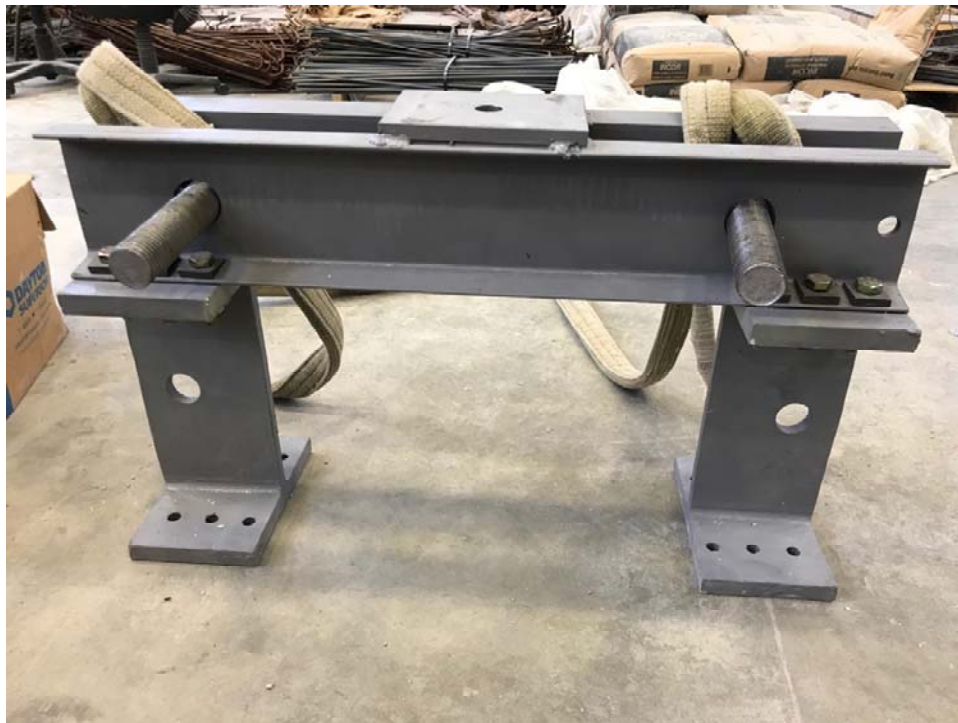
Figure 3.10: Load frame used for unconfined tests
