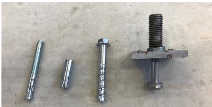
Figure 1.1: Examples of common anchor types (from left to right: torque-controlled, displacement-controlled, screw, and cast-in anchors)
