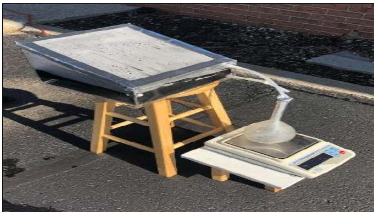
Figure 17 Produced Water evaporation using natural solar light.
