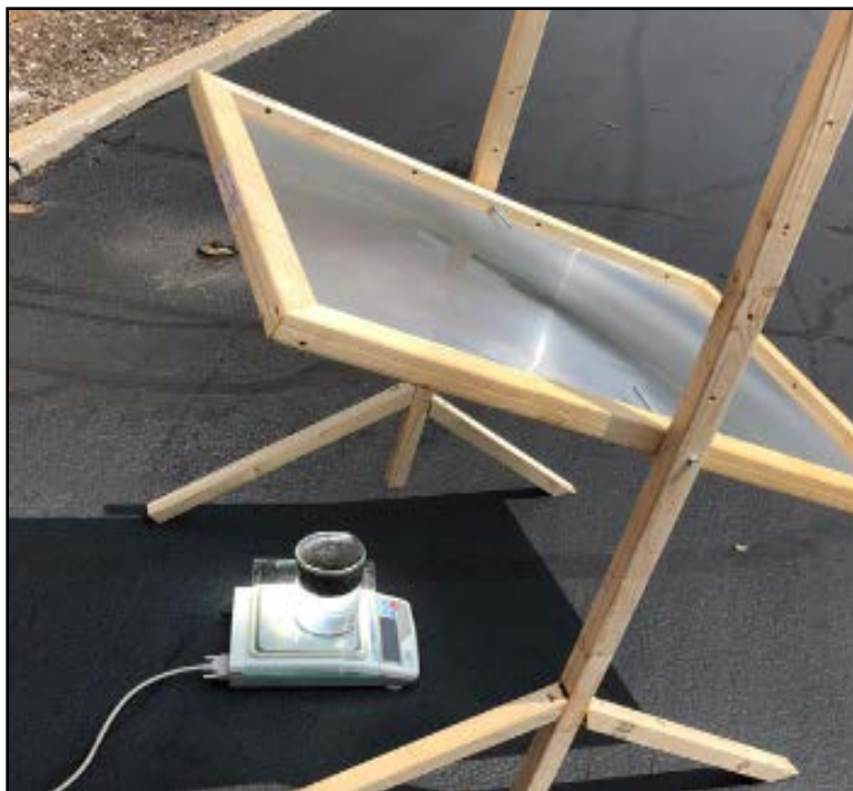
Figure 15 Steam generation using fresnel lens.
