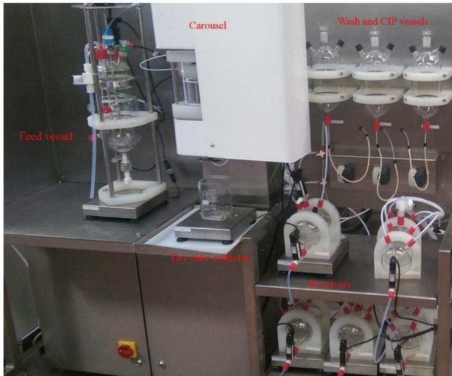
Figure 2-34 A continuous filtration drying unit developed by AWL. Permission obtained from [147] Copyright © 2019 American Pharmacists Association® Published by Elsevier Inc.
