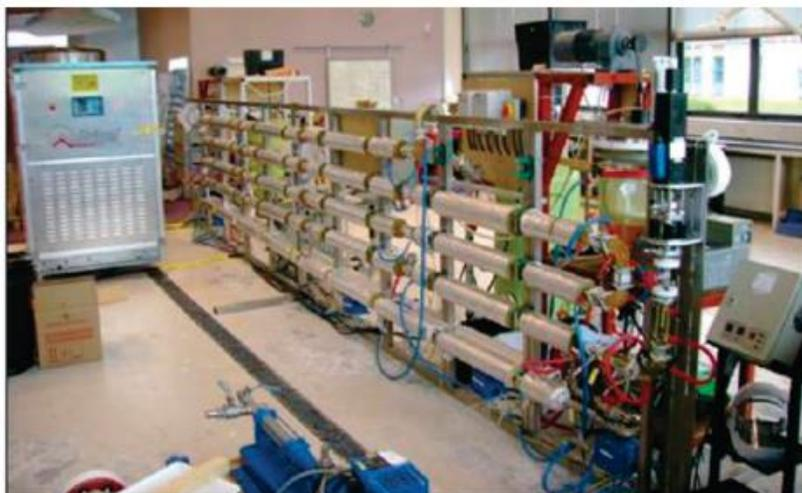
Figure 2-30 A custom built stainless steel OFBC unit. Permission obtained from [133] Copyright © 2009, American Chemical Society.
