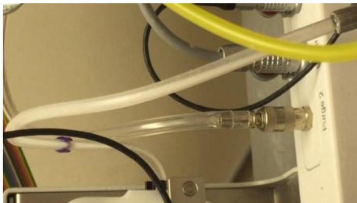
Figure 2-23 A blocked slurry transfer line of a lab scale MSMPR. Permission obtained from [23] Copyright © 2017, ACS.
