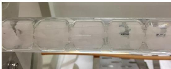
Figure 2-28 Image of an encrusted tube section of a tubular PFC.
