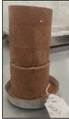
Figure 4-22. Collapse of a High Plasticity QL Treated Sample During Wetting/Drying Cycles
