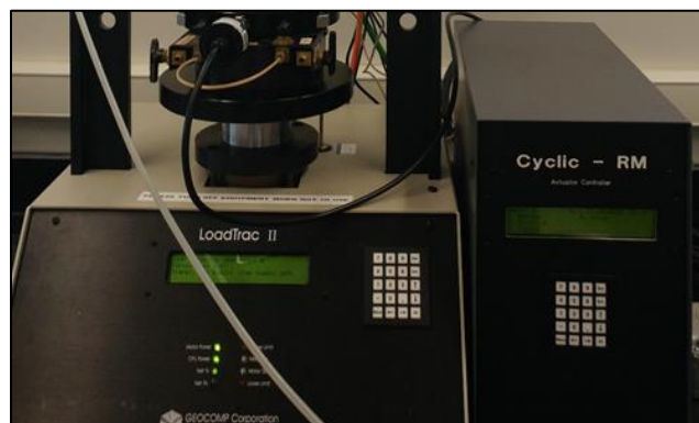
Figure 4-18. LoadTrac-II/Cyclic-RM and Load Frame (INDOT laboratory)
