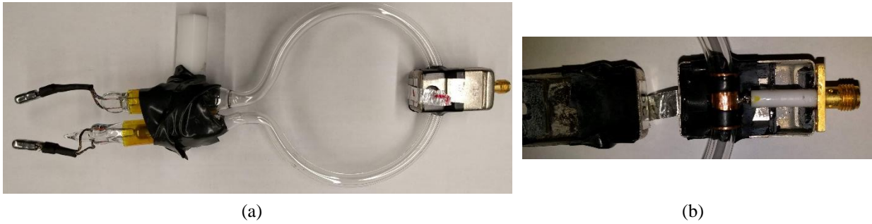
Figure 7.4. (a) coupler mounted to the plasma antenna and (b) the internal structure of the coupler.
