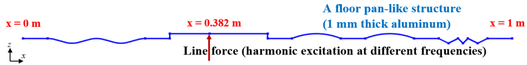
Figure 7.11. A 1 mm thick, harmonic line force-driven, arbitrarily-shaped aluminum panel to model a vehicle floor pan-like structure.
