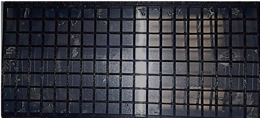
Figure 20: Wick support, top view. The openings allow for downward vapor displacement to the Aluminum wall of the heat sink, without compromising the structural integrity of the support in maintaining uniform contact between the wick and the TEGs.
