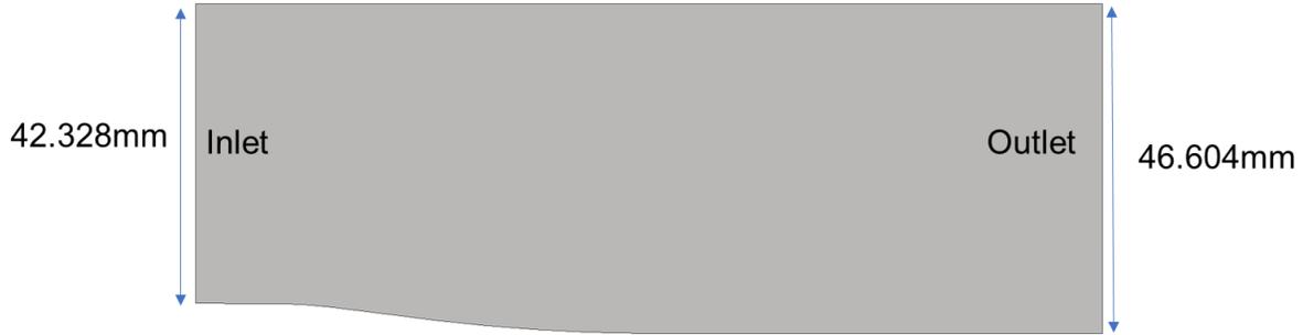
Figure 75. Channel geometry without stator, rotor, or purge
