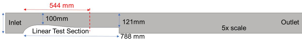
Figure 76. Test Article 5x scaled
