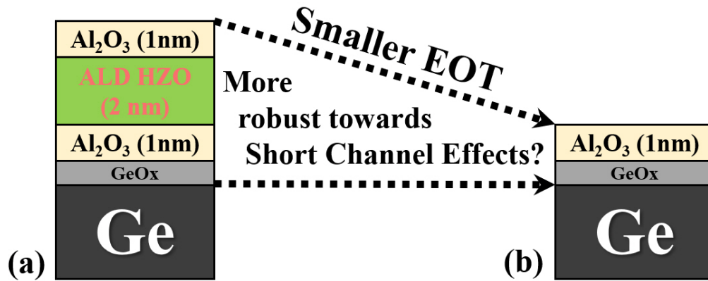
Fig. 3.9. Gate stacks of (a) germanium NC FinFETs and (b) reported germanium FinFETs using the same fabrication process and equipment [15].
