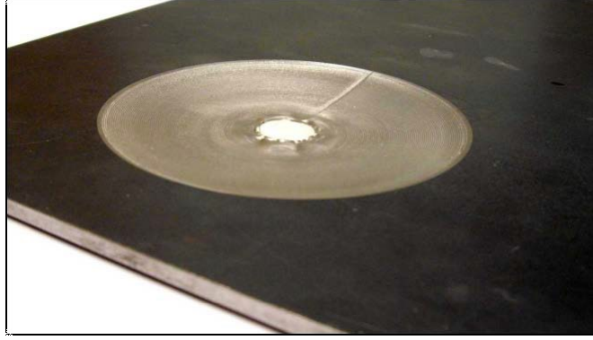
Fig. 2.3.: A 2D acoustic black hole in the form of circular indentation for flexural wave attenuation. Adapted from [72]. (Copyright Victor V. Krylov)
