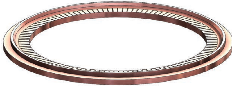
Figure 2.17. CAD render of injector insert with 120 injectors, groove width 0.38 mm (0.015 in).
