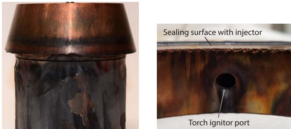
(a) Centerbody showing extensive melting and charring. Image courtesy of Jenna Humble.
