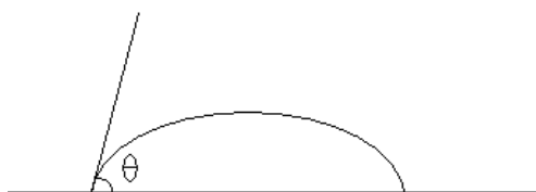
Figure 4: This figure shows an example of how a contact angle is measured.
