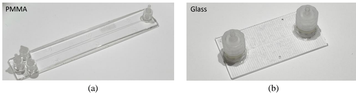
Figure 5.2. Photographs of the microfluidic chips used in the test: (a) PMMA and (b) Fused silica glass. Two of the three holes at the exit of PMMA channel are blocked using mini-luer plugs.
