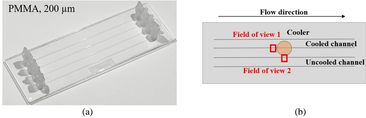
Figure 5.11. (a) Image of the PMMA chip with four parallel channels and (b) schematic diagram showing the location of the fields-of-view with respect to the cooler contact region.
