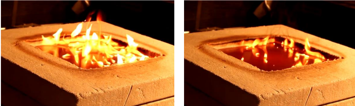
Figure 3-23: Test fuel flame image – distributed ignition at 840°C set temperature
