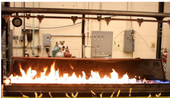
Figure 7-3: Flame front image for 70°C (left) and 90°C (right) initial HEFA-50 fuel temperatures at identical times
