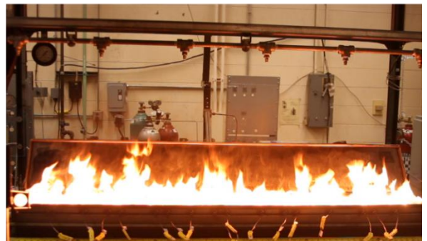
Figure 7-3: Flame front image for 70°C (left) and 90°C (right) initial HEFA-50 fuel temperatures at identical times
