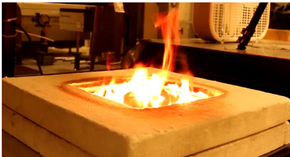
Figure 3-28: Test fuel D flame image – distributed ignition at 810^{\circ}\text{C} set temperature
