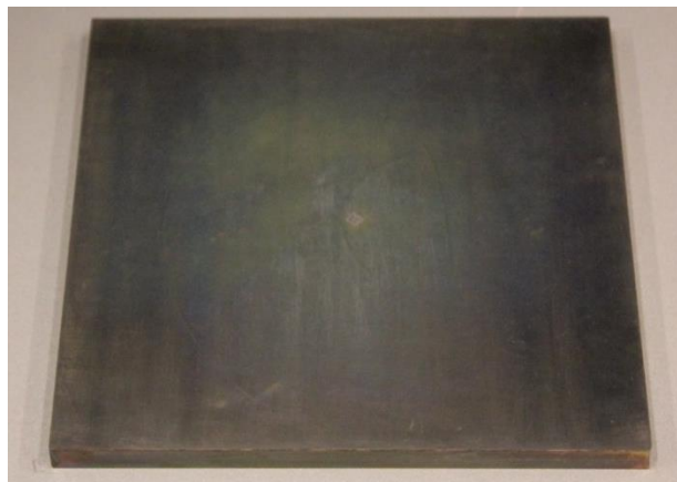
Figure 3-31: Plate after ignition tests – baseline fuel Avgas 100LL
