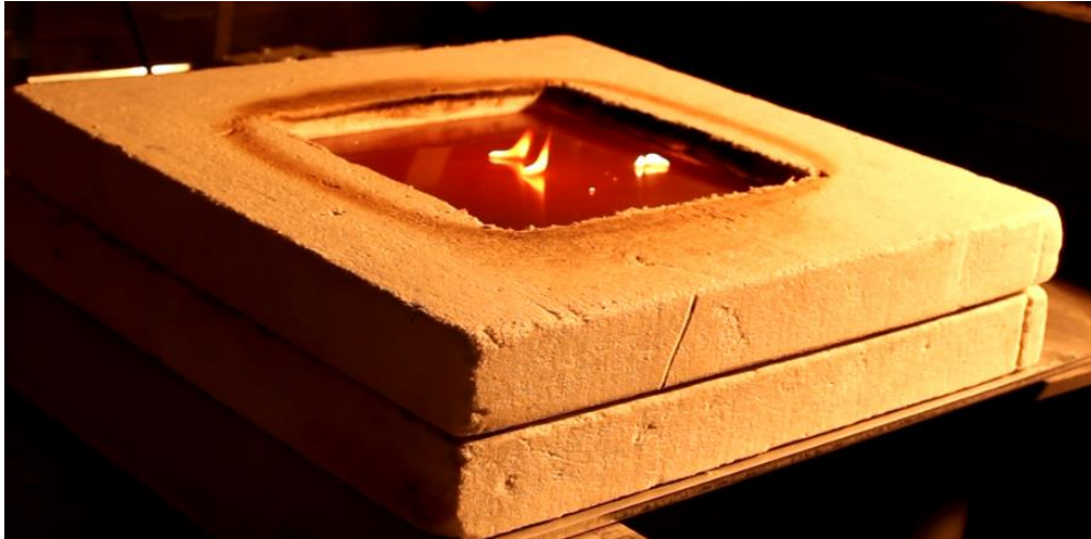
Figure 3-11: Point ignition at 890°C surface temperature
