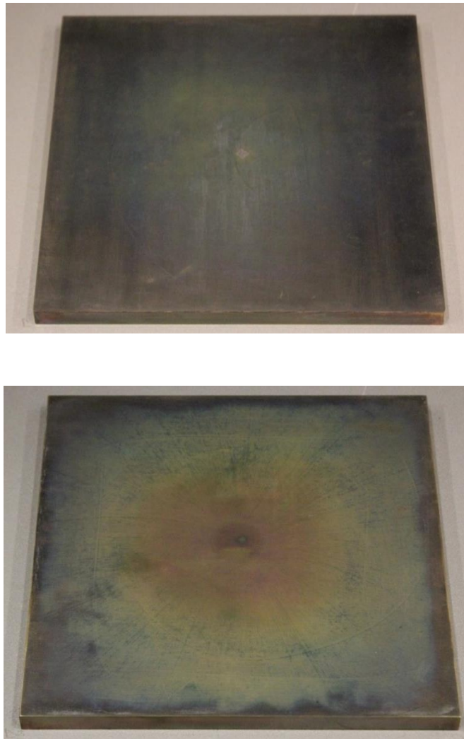
Figure 3-26: Plate after ignition tests – baseline fuel ( top ) and test fuel C ( bottom )
