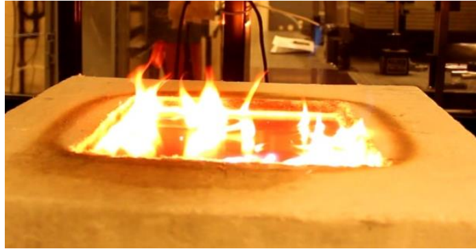
Figure 3-8: Baseline fuel flame image at 810°C set temperature
