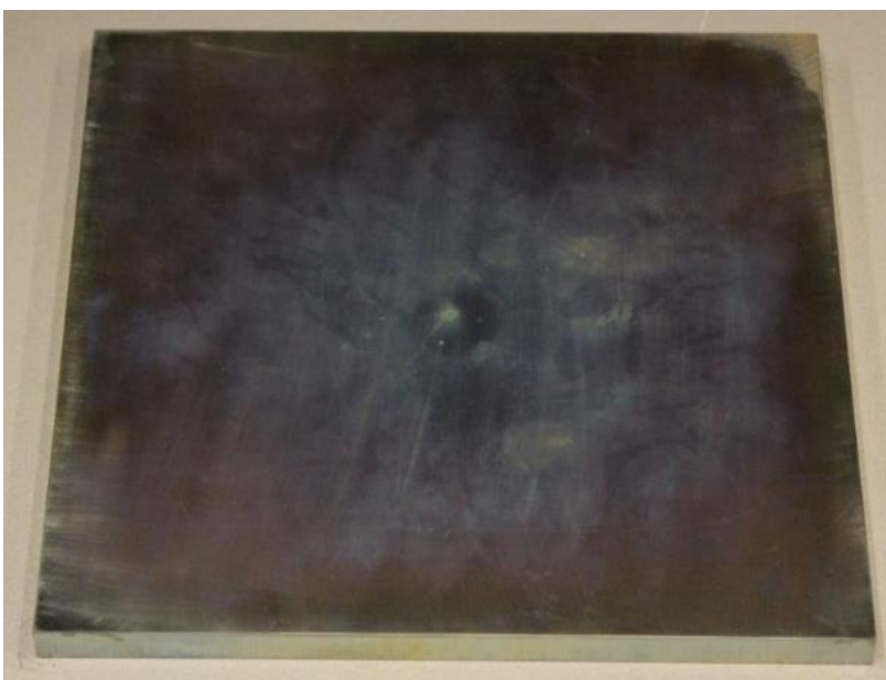
Figure 3-21: Plate after ignition tests – test fuel B
