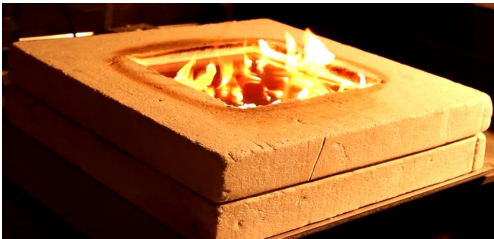
Figure 3-12: Distributed ignition at 900°C surface temperature
