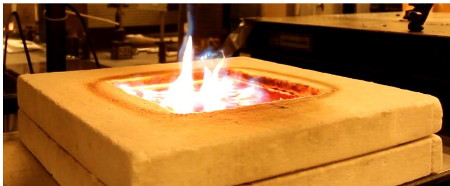
Figure 3-17: Test fuel flame image – distributed ignition at 770^{\circ}\text{C} set temperature
