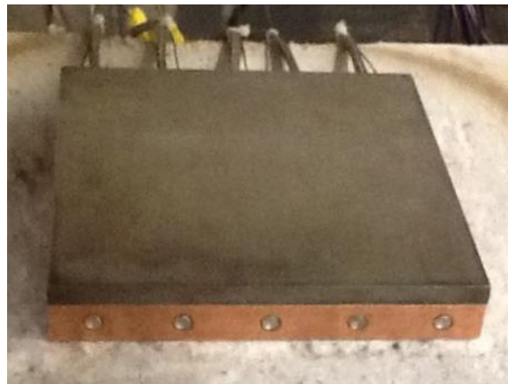
Figure 2-2: Stainless steel plate bolted to the copper plate assembly containing five 1000 W cartridge heaters
