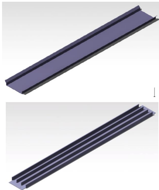
Figure 5-6: CAD models of top test pan ( top ) and bottom ( bottom ) pan
