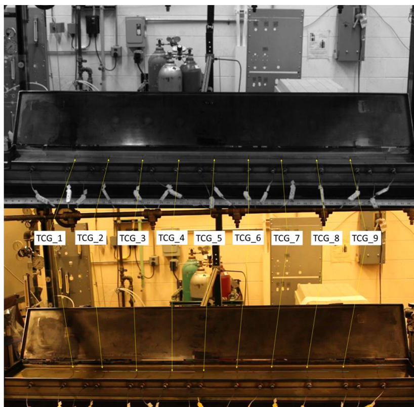
Figure 6-1: Gas-phase thermocouple locations
