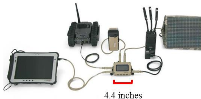
Figure 2.4. SPM-622 harvesting power to charge military equipment. [34]
