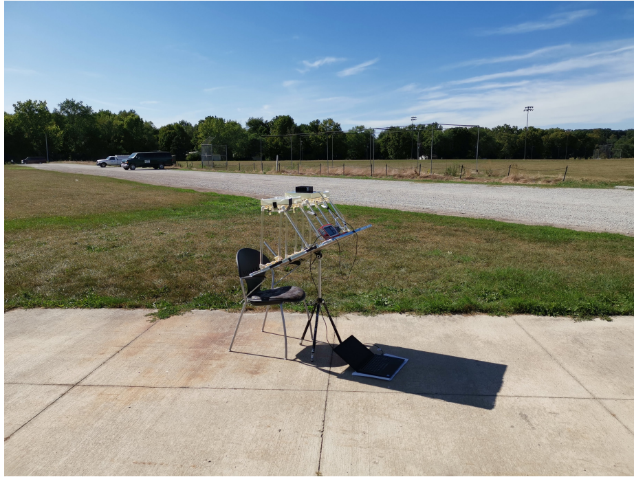
Fig. 4.6. The surface albedo is a combination of reflection mostly from wood board, concrete, grass, and rock roads. The albedo of grass is typically \sim 0.26 , the white concrete and rocks can be higher than 0.6. The estimated average albedo in simulation is 0.35.
