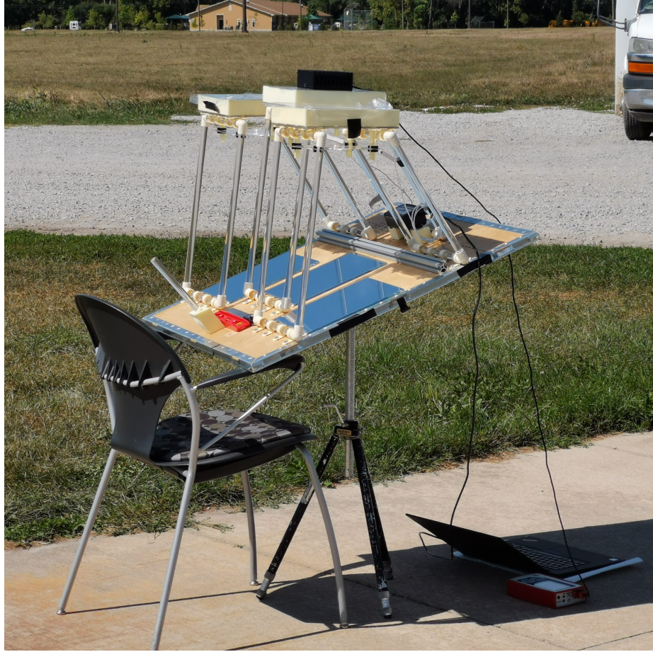
Fig. 3.1. Aligned experiment setup during outdoor test. Specifically, Avg. Solar Power indicates the average solar irradiance during the entire experiment measured by thermal sensor; \Delta T is the steady-state temperature difference of chamber 1 and 2; \Delta V_{OC} is the steady-state open-circuit voltage difference of solar cells in chamber 1 and 2
