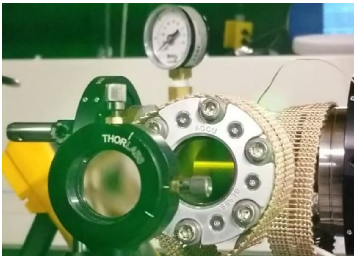
Fig. 5.5. Constructed calibration cell showing I_2 fluorescence.
