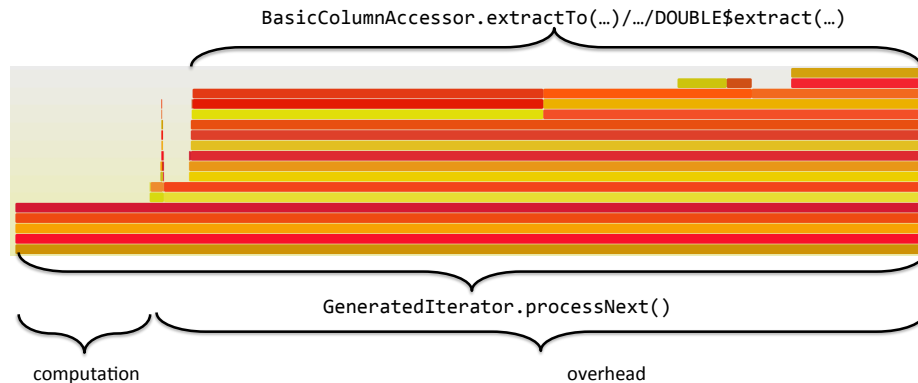
Figure 2.6.: CPU profile of TPC-H Q6 in Spark SQL, after preloading the lineitem table. 80% of time is spent accessing and decoding the in-memory data representation.
