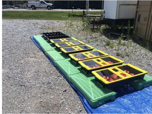
Figure 3.2. Dehytray™ arrangement when placed under the sun during drying studies.
