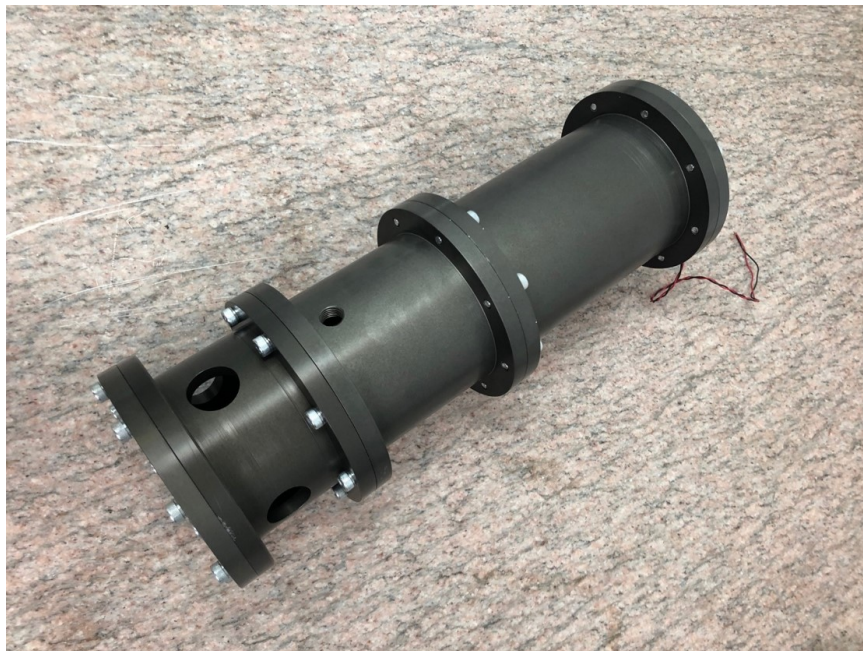
Fig. 6.60. Picture of the final version of the prototype linear compressor.
