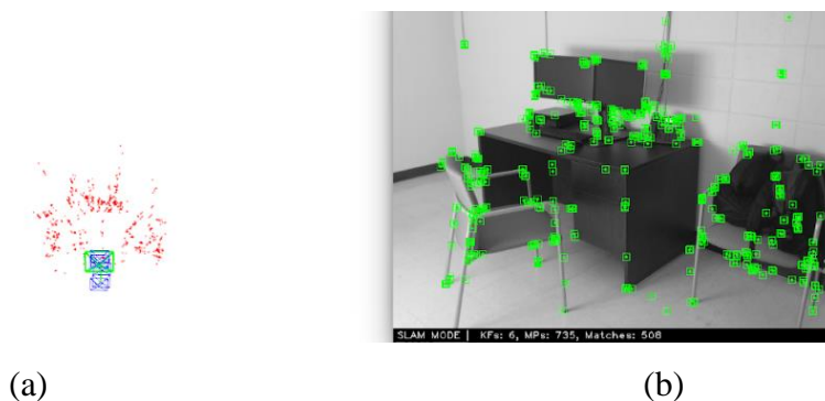
Figure 4.6. Numbers of feature points found and matched. Red dots in (a) shows the corresponding green features from (b). Green frame in (a) is the current camera position in the map.
