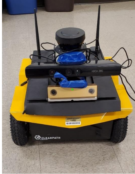
Figure 4.2. The Jackal mobile robot mount with both Bumblebee camera and RGB-D camera.
