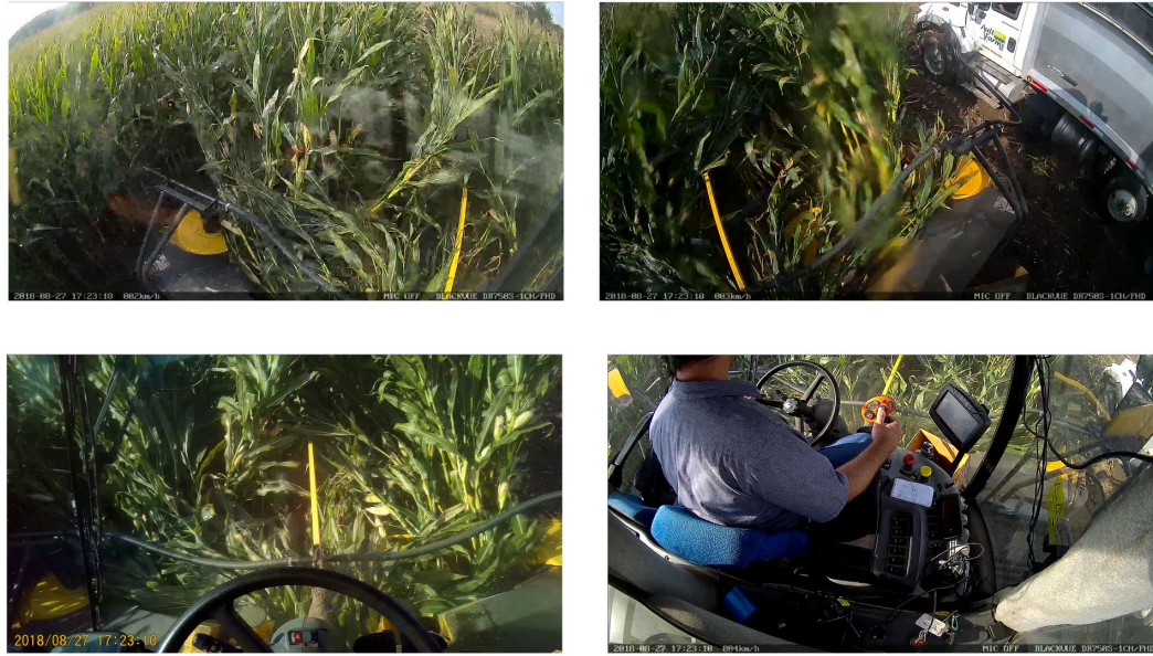
Figure 2.1.: Different video angles from the camera system installed in a corn chopper. The upper two images show the sample images from the two dash cameras on the left and right side. The bottom left image is captured by the nose camera. The bottom right camera is placed at the back window to capture the actions of the operator.
