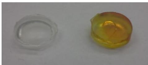
Figure 4.5. Untouched epoxy pellet (left) compared to epoxy pellet after being contacted with WFNA and rinsed with DI water (right).
