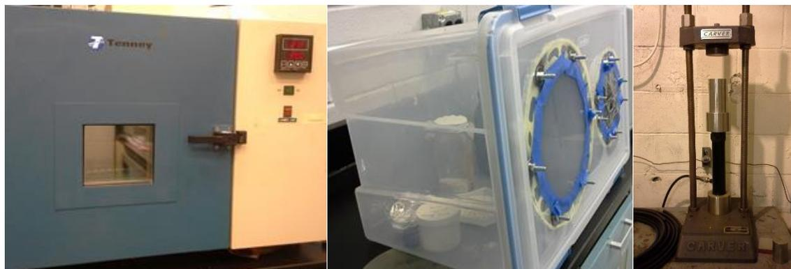
Figure 3.1. Equipment used for fuel pellet preparation: oven (left), dry box (center), and Carver press (right).
