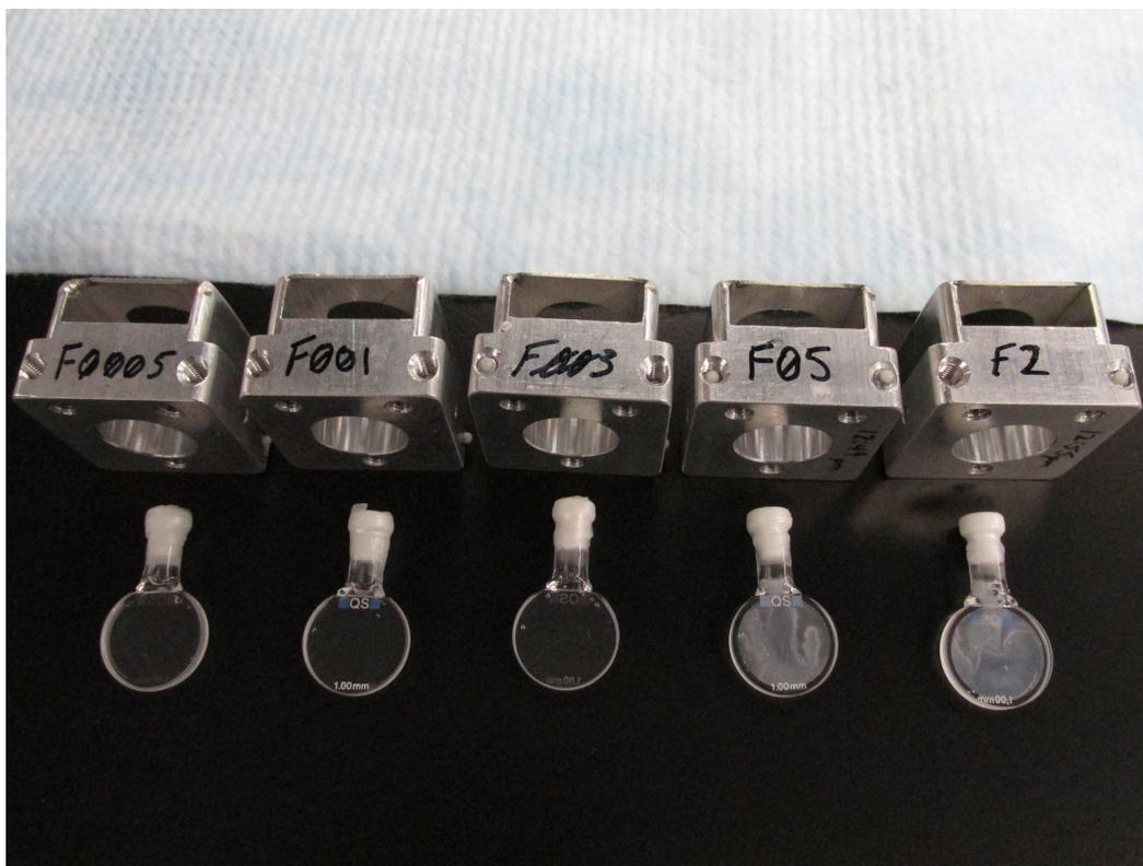
Fig. 3.3. Examples of loaded fibrinogen (4.78 mg/ml) with thrombin (in concentrations of 0.005, 0.01, 0.03, 0.5 and 2.0 unit/ml; from left to right) samples into the banjo (quartz) holders for SANS measurements.
