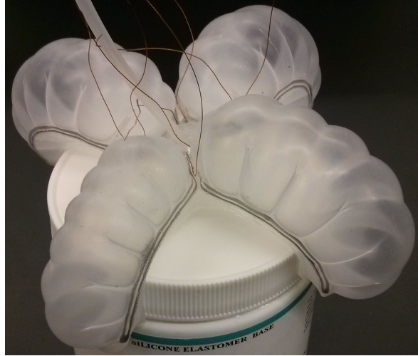
Figure 2.5. The pneumatic robot gripping a cylindrical container. The serpentine liquid-metal sensor channels are clearly visible around the outside edges of the pneumatic channels (dark against the white background).
