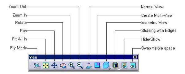
Figure 1.3 Viewing tools in Catia(A CAD package)
