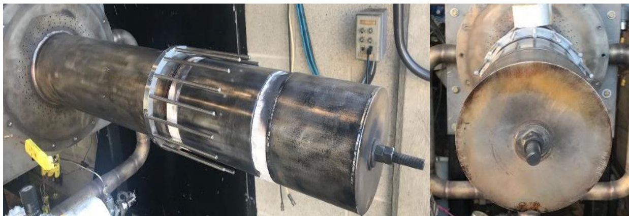
Figure 3-13 Claw obstacle installed at position 1 (P1) on the test apparatus
