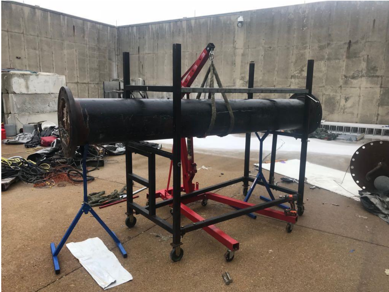
Figure 2-5 Exhaust tube in construction for test fluid waste capture system in courtyard behind test facility (HPL, Zucrow Laboratories)
