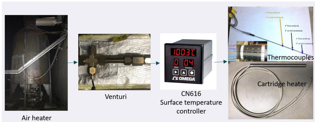
Figure 2-17 Test procedure and experimental technique
