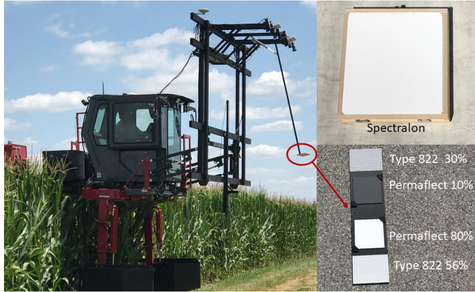
Figure 3.5. Calibrated targets on PhenoRover and Spectralon 98% used as white reference.
