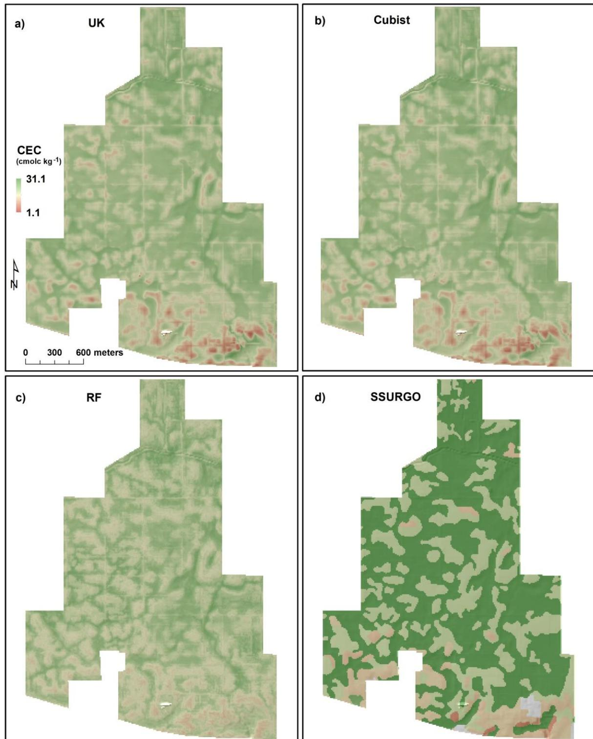
**Figure 3.7:** Cation exchange capacity (CEC) prediction. a) Universal kriging (UK), b) Cubist, c) random forest (RF), and d) soil survey geographic (SSURGO).
