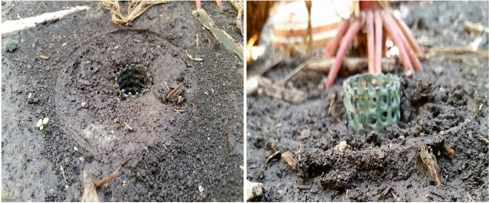
Figure 3-15. Representation of perforated cylinders from the soil surface where one image (left) shows a properly installed cylinder that is even with the soil surface and the second image (right) shows a poorly installed cylinder. Cylinders installed a few cm above the soil surface (right) were forced into the ground during installation until even with the soil mounds that were created at the soil surface after drilling with the augur bit. Once the mound of soil around the top of the cylinders had settled, it was revealed that the cylinders were actually a few cm above the soil surface. Roots growing at 0-5 cm deep, for example, would have then penetrated the cylinder void at the 5-10 cm painted markings.
