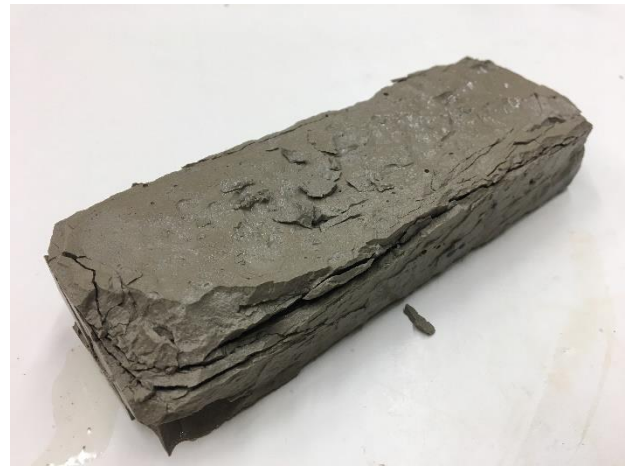
(b) AE CSC paste at 160 F/T cycles
