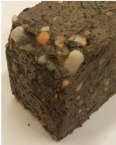
(c) AE CSCC-pea gravel at 150 F/T cycles
