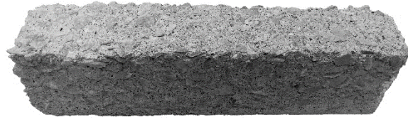
(b) AE reference concrete after 992 cycles
