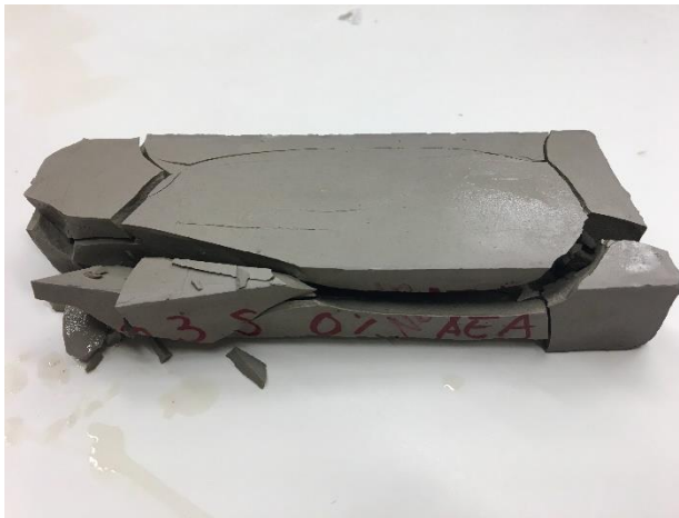
(a) non-AE CSC paste at 4 F/T cycles
