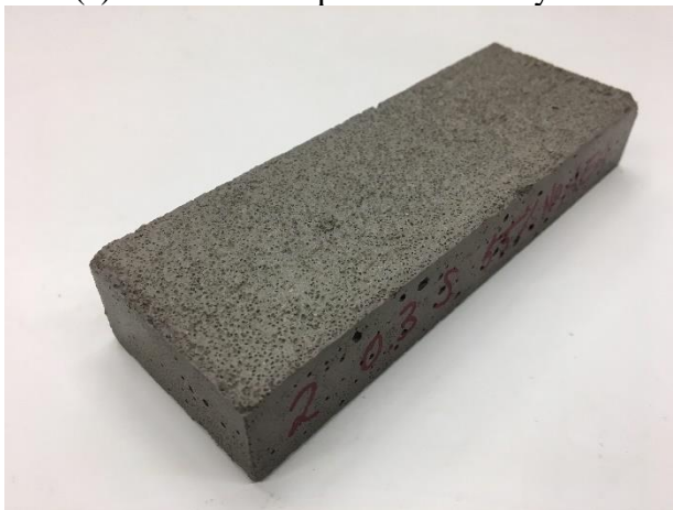
(c) non-AE CSC mortar-55% agg. at 36cycles
