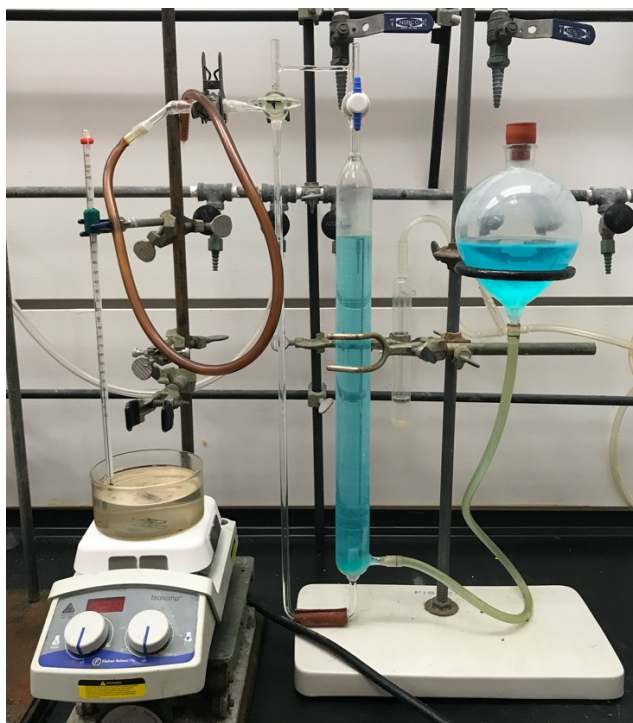
Figure 2.4 Hydride apparatus with oil bath and hot plate for heating/stirring
