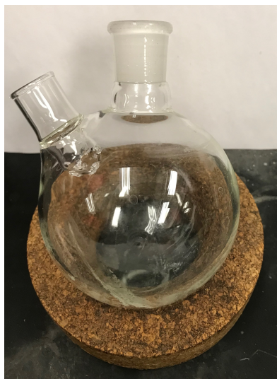
Figure 2.3 Custom dry ice reaction flask with refillable, “porous,” and sealable side-arm
