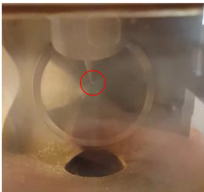
Figure 4.2 Photograph of the plasma discharge during an ethanethiol experiment with a negative mode ESI voltage of 3 kV and an ethanethiol flow rate of 10 \mu\text{L}/\text{min} . The plasma discharge is located at the tip of the ESI needle and is in the middle of the red circle (added for emphasis).
