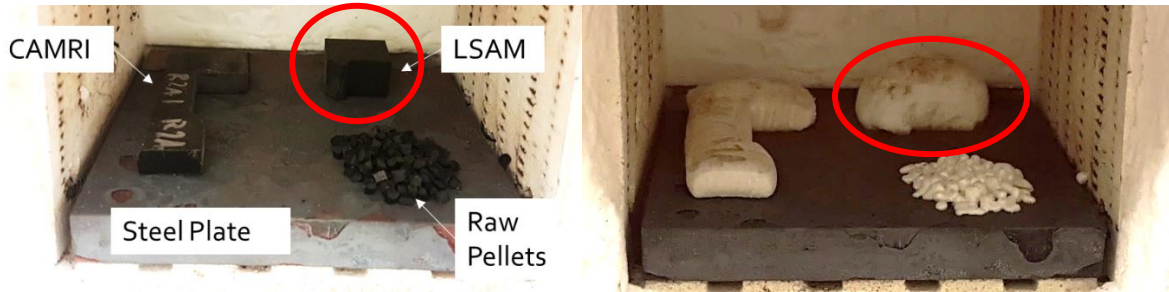
Figure 2.2-3: Printed GF-PA before and after burning off the matrix
