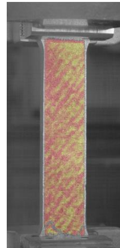
Figure 2.3-5: Example plot of the transverse versus axial strain measured by Digital Image Correlation used to determine the Poisson Ratio
