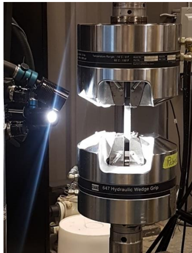
Figure 2.3-6: Tensile test setup for the tensile test in the 2 and 3-direction
