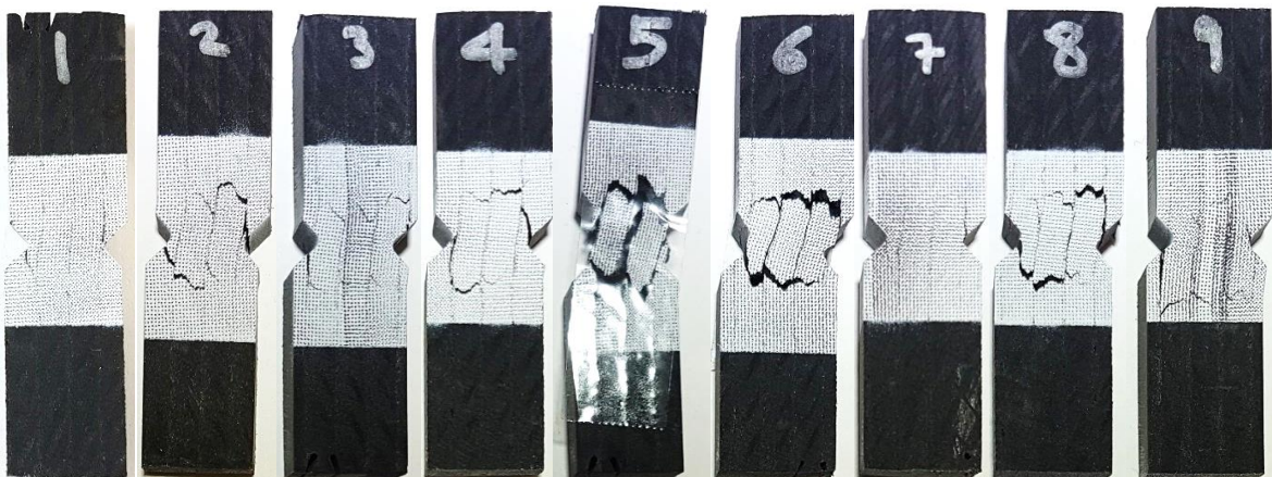
Figure 2.3-18: Fractured shear specimens
