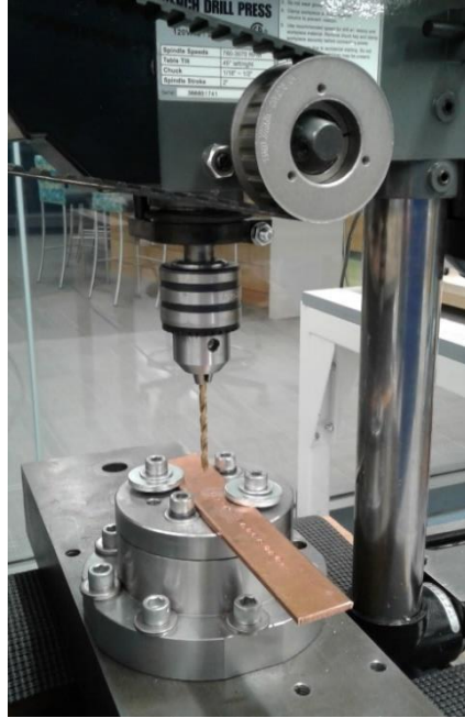
Figure 4.19. Experimental setup for the drilling of Cu. A benchtop drill press was modified to provide a controllable, constant feed rate. Cu workpiece mounted atop a piezoelectric dynamometer to measure thrust force and torque.
