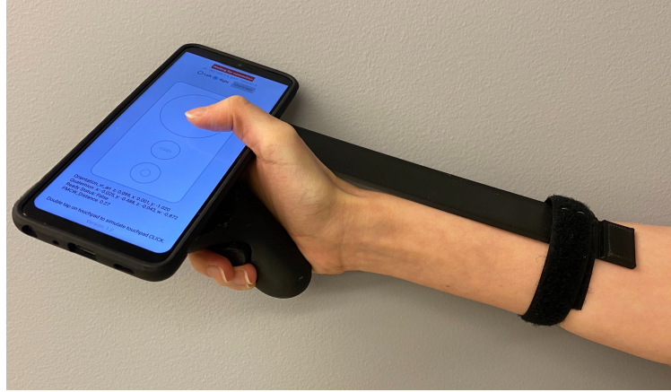
Fig. 4.10. 3D printed controller used in VIU .
