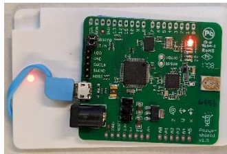
Figure 4.1. Pozyx tag placed in OR personnel's pockets for location positioning
